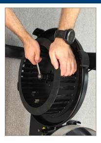
5. Install the new "turbo" flywheel and tighten the flywheel axle nuts with the 2x 9/16" or 15 mm wrenches.
