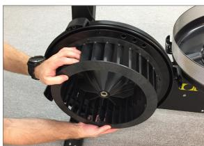
Using a small Philips screwdriver, remove the old wire cover from the inside of the flywheel housing and install the new wire cover with supplied screws.
